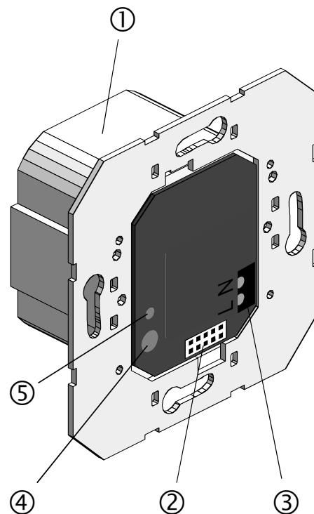
This device is provided for installation into 60 mm standard flush boxes. Flush-mounted mains coupler ① must be fixed solely by the supporting ring in connection with the screws on the flush box. User interface (AST) ② must be below.
