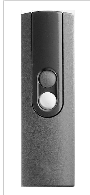
Irrespective of the programming performed during the installation, the radio hand transmitter can be used for internal or external arming/unarming. Moreover, operation as pure remote control for switching on or off a consumer connected to the radio alarm center or radio sub-center is possible. The flush-mounted control key and the pressing period of 1 s avoid unintentional actuation.
