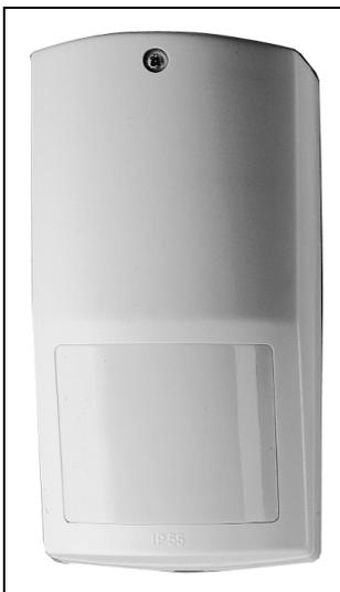
Due to specific optics (a so-called Fresnel lens) fan-shaped observation of the space within a detection range of 8 x 11 m (90°) is possible for an installation height of 2.4 m.
