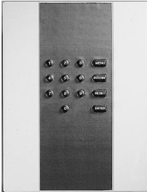
Via the keyboard of the radio door module, the radio alarm center can be internally or externally armed or unarmed after previous code entry. A specific "CODE" function key allows the user's code to be changed.
