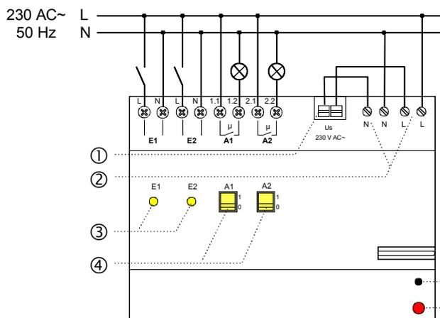
**Switch off the mains voltage prior to establishing the electrical connection.** Establish electrical connection as shown in the opposite illustration.
