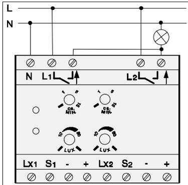
Connection of all system sensors on one load (time and lux setting separately per channel).
