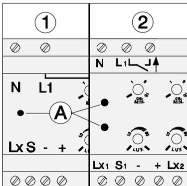
The optical displays (A) of the System Power Booster REG 1channel ① respectively 2channel ② signalise the switching-on of load.
