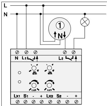
Example for application with time switch clock ① (clock with 230 V switching output).
