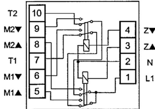
**Parallel connection of cut-off relays**
