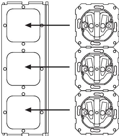
9. Hang the device carrier in the device box on the side (with two device carriers) or in the centre (with one device carrier).
