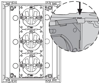
10. Connect the flush-mounted inserts and fold the device carrier closed.
