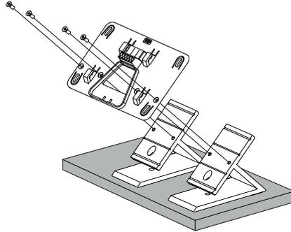
2. Guide the supply cable through the rear cover plate and the mounting plate.
