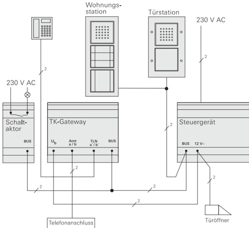
The single-family house has a door station, a home station with an additional call button, a switching actuator, which is to switch the outside light, and a TC-gateway. The TC-gateway is connected to the analogue telephone connection.
