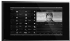
The Gira Control 19 Client is a PC-based control and regulation unit with a brilliant, capacitive touch screen with a screen diagonal of 47 cm (18.5"). Thanks to the integration of a loudspeaker and microphone and in combination with the Gira DCS-IP-gateway, the Gira Control 19 Client can also be used as a home station for audio-visual door communication.
