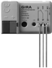
The flush-mounted DCS switching actuator carries out switching functions via its zero-voltage relay contact (24 V SELV, 50  $\mu$ A to 1.6 A AC/DC) which are triggered via the 2-wire bus.
