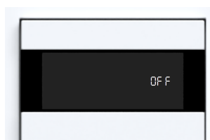
Figure 18: Display in switched-off state
