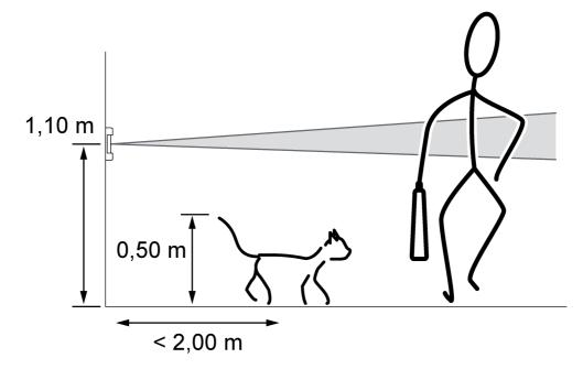
Figure 11: Detection field and mounting height
