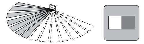
Figure 12: Limiting the detection area
