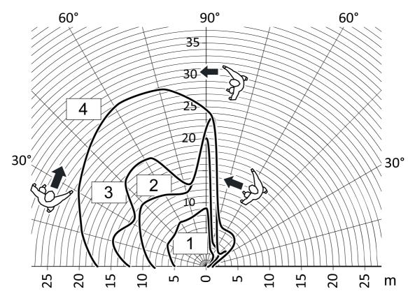
Figure 13: Range with tangential direction of motion
