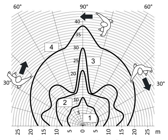
Figure 9: Range with tangential direction of motion
