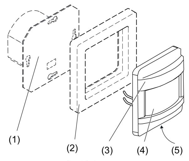
Figure 1: Device components
