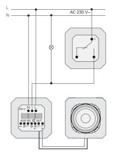
If no permanent phase exists in the room, connection of the flush-mounted radio can alternatively be carried out via the switched phase. In this case however the flush-mounted radio may only be operated with lighting switched on.
