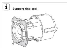
The support ring of the loudspeaker insert is coated with a film that provides acoustic isolation of the insert from the front sound opening. This support ring seal must not be removed and, apart from holes caused by the attachment screws must not be damaged, as otherwise bass reproduction may be impaired.
