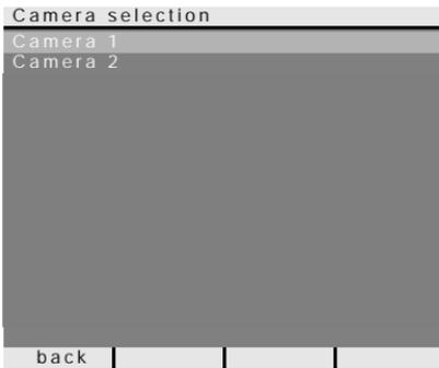
In the "Camera selection" menu all assigned colour cameras are displayed. The desired camera can be selected and switched on by turning and pressing the operating button.
