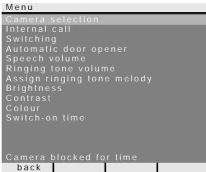
If the menu item "Camera selection" is selected while a "video conversation" is in progress in the door communication system, "Camera blocked for time" appears in the status line.
