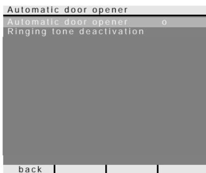
The automatic door opener is activated or deactivated by turning and pressing the operating button.
