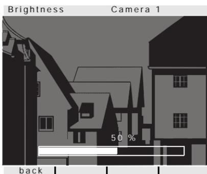
In the "Brightness", "Contrast" or "Colour" menu, the respective parameters can be selected and set by turning and pressing the operating button.
