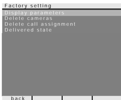
Here the settings of the VideoTerminals are reset to the factory settings.
