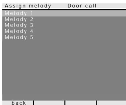
In the "Assign melody" menu the melody of the last ringing tone triggered can be selected by turning and pressing the operating button.
