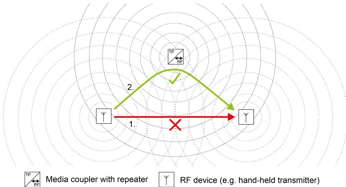
Image 6: Application example of a media coupler with repeater function
