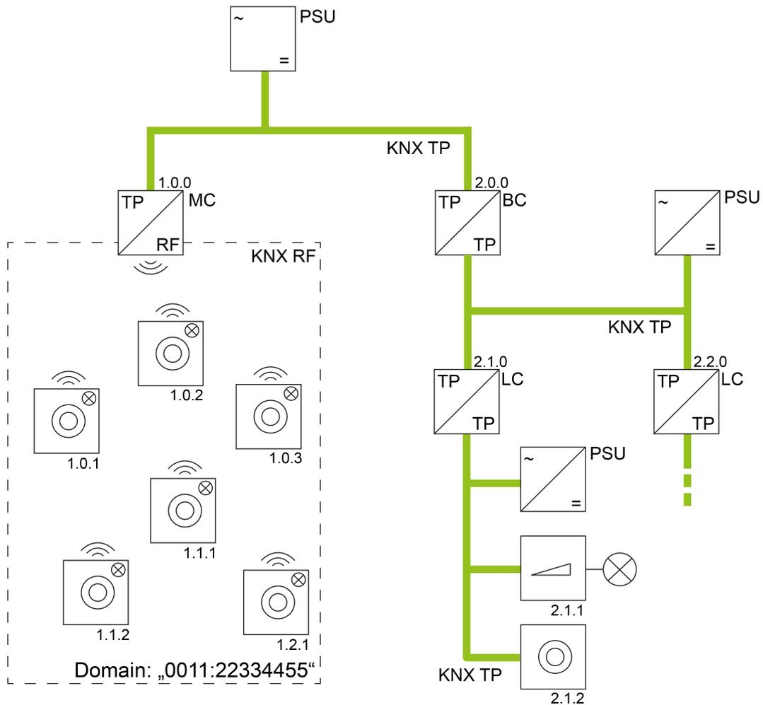
Image 2: Example of a possible KNX topology with RF and TP lines
