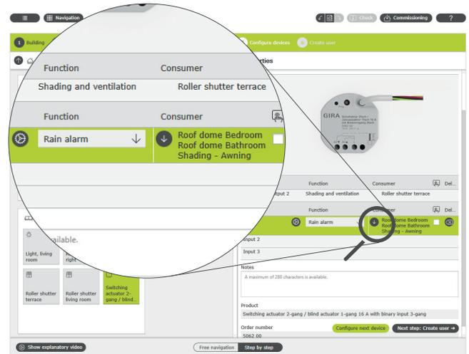
Assigning several devices to the "Rain alarm" function
