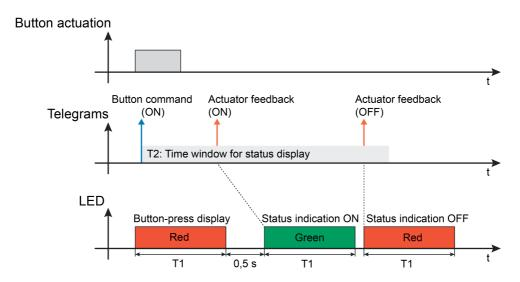
Figure 9: Example of a two-level actuation and status display with double status Reception of two actuator status messages in time window permitted
