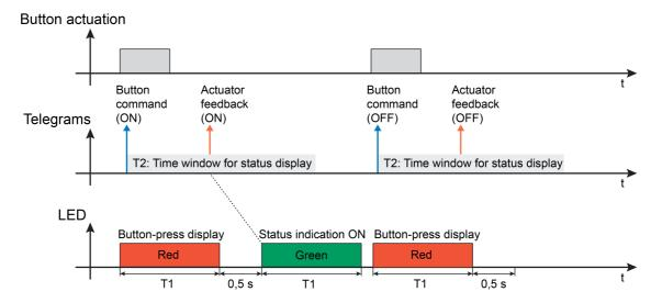
Figure 5: Example of a two-level actuation and status display with single status Status display state "ON" through green LED
