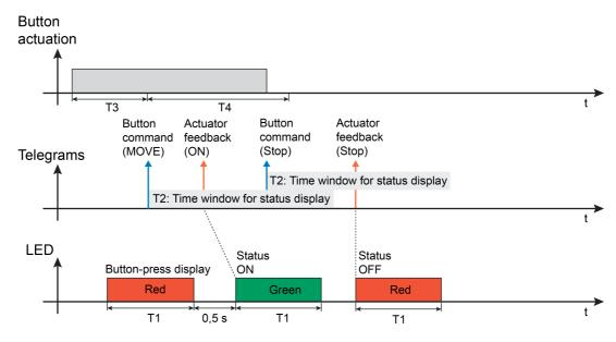
Figure 19: Example of a status display with the operating function "Venetian blind" with a long button-press
