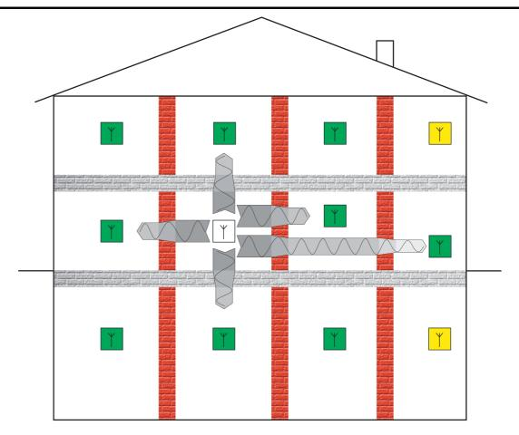
Figure 28: Attenuation of the radio signal in buildings through walls and ceilings Example 2: "Central position of the transmitter" (simplified depiction)
