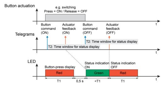
Figure 8: Example of a two-level actuation and status display with double status Interruption of the first status display through the actuator status in the new time window
