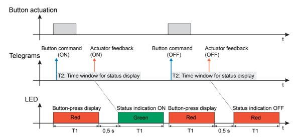
Figure 6: Example of a two-level actuation and status display with double status Status display state "ON" and "OFF" through green and red LED
