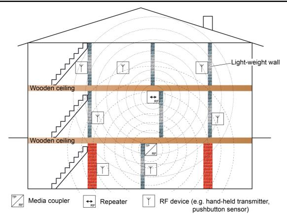
Figure 36: Building structure with one KNX RF line and repeater (example)
