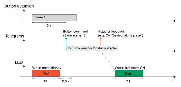
Figure 22: Example of a status display with the operating function "Scene extension" Scene extension with memory function and status display (with single status ON)
