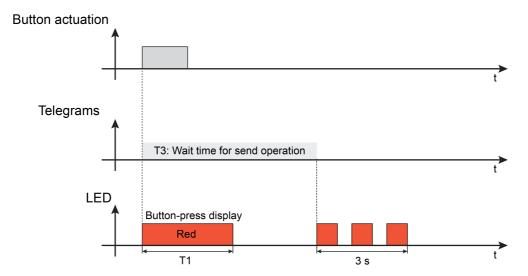
Figure 12: LED display in the case of a transmission error
