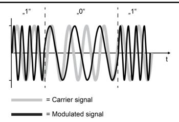
Figure 26: Frequency key shifting as a modulation method (FSK = Frequency Shift Keying)
