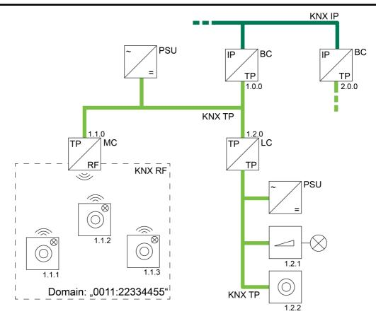
Figure 39: Example of a possible KNX topology with RF, TP and IP lines Media coupler as line coupler
