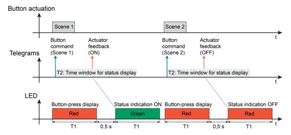
Figure 21: Example of a status display with the operating function "Scene extension" Scene extension without storage function (with double status ON and OFF)
