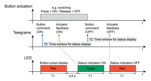
Figure 7: Example of a two-level actuation and status display with double status New time window for status display through multiple operating telegrams
