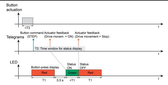
Figure 18: Example of a status display with the operating function "Venetian blind" with a short button-press (with double status ON and OFF)
