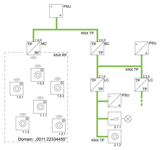
Figure 40: Example of a possible KNX topology with RF and TP lines Media coupler as backbone coupler
