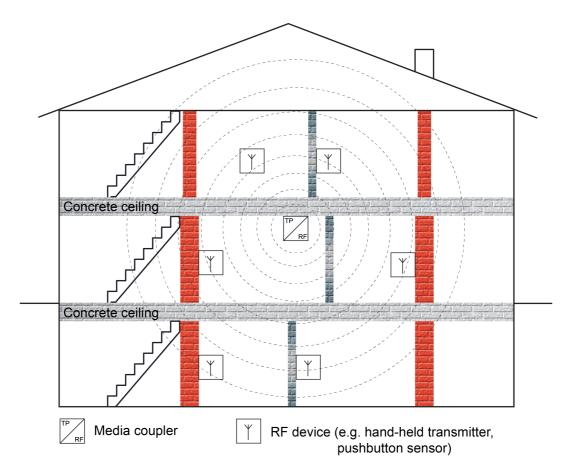
Figure 34: Building with a KNX RF line (example)
