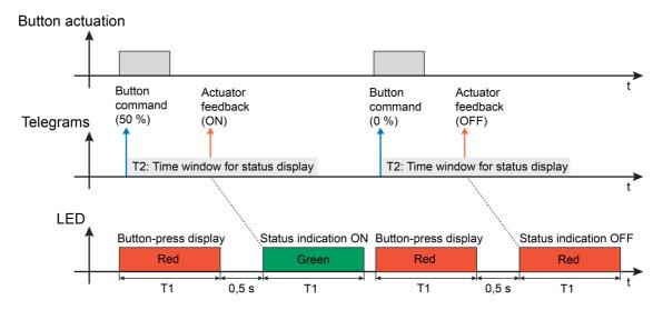
Figure 20: Example of a status display with the operating function "Value transmitter 1-byte" with double status (ON and OFF)
