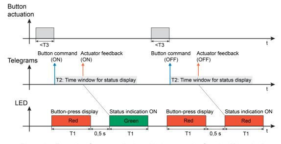
Figure 15: Example of a status display with the operating function "Dimming" with a short button-press (with double status ON and OFF)
