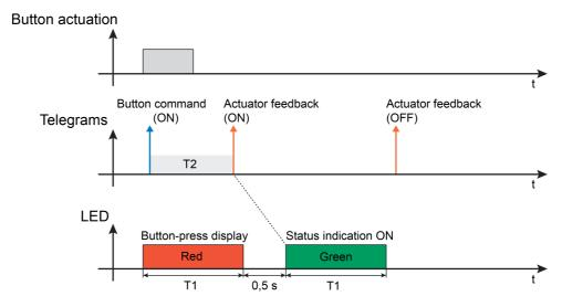
Figure 10: Example of a two-level actuation and status display with double status Reception of two actuator status messages in time window not permitted
