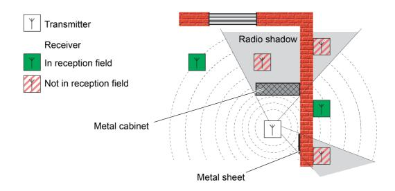
Figure 30: Radio shadow in a building due to metallic parts (idealised)
