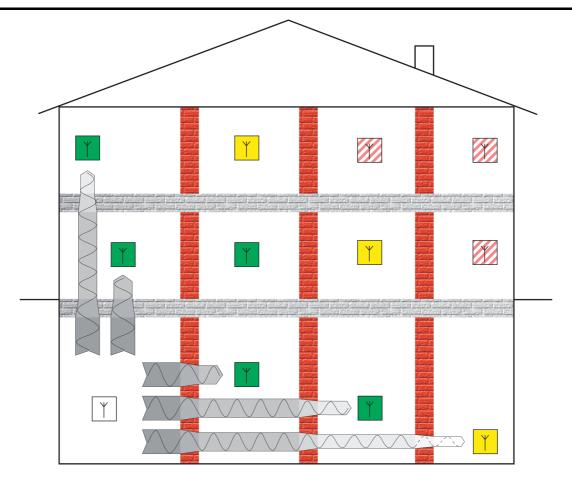
Position of transmitters (e.g. hand-held transmitter, pushbutton sensor)
