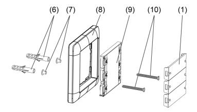
Figure 2: Screw mounting
