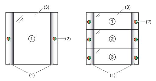
Figure 1: Device components Push-button sensor, 1-gang (left) and 3-gang (right)
