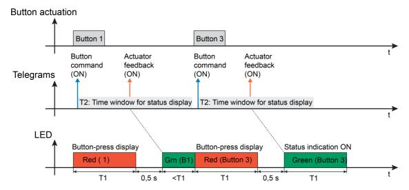
Figure 11: Example of a two-level actuation and status display Interruption of the display function through new button actuation
