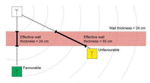
Figure 29: Attenuation through effective wall or ceiling thickness
