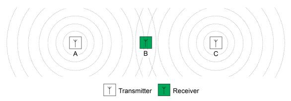
Figure 24: Radio collisions on the receiver due to the transmitter being too far away
