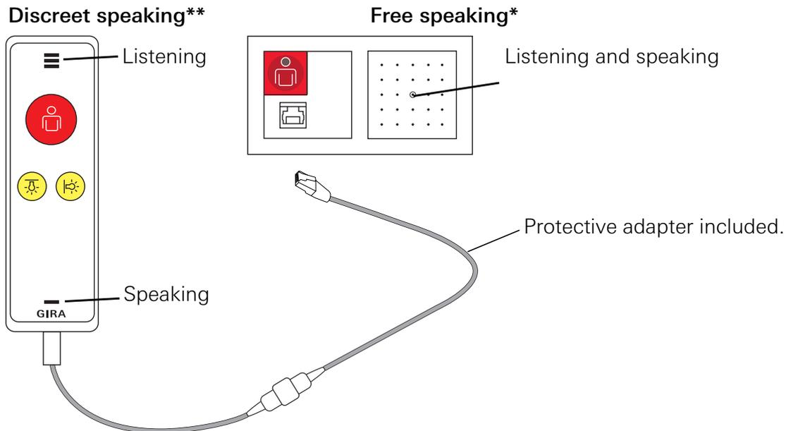
Figure 3.10: Connection between the patient hand-held device and the room device with ancillary plug contact
