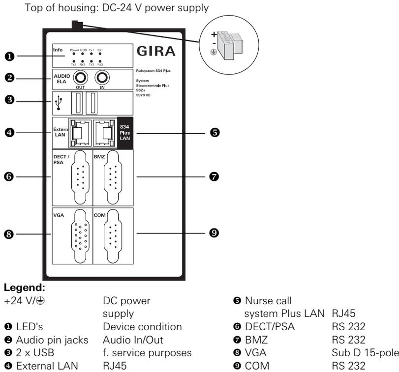
Figure 3.29: Connections of the system central control unit
