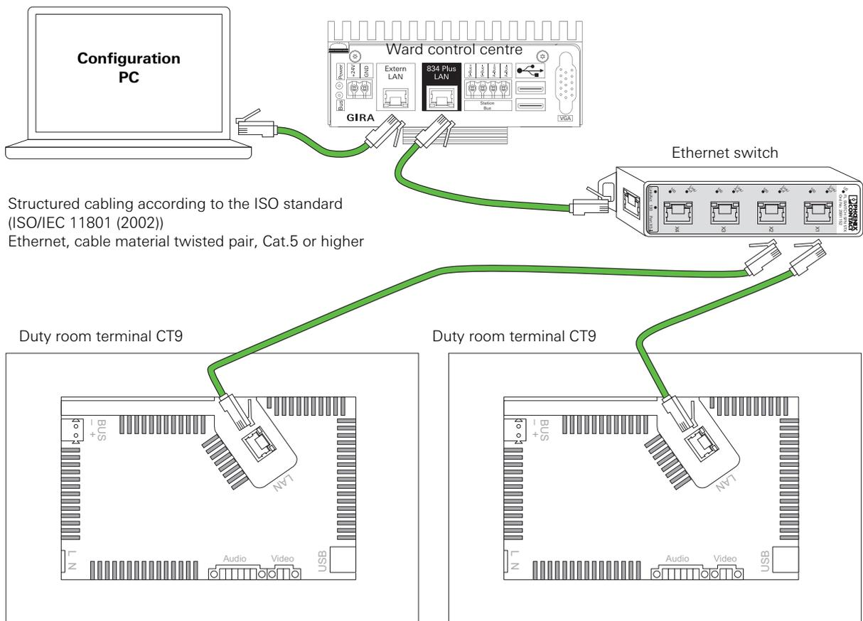
Structured cabling according to the ISO standard (ISO/IEC 11801 (2002))
