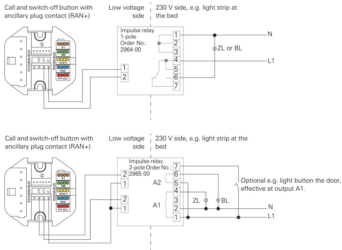
Figure 3.11: Connection of room light (ZL) and/or bed light (BL)
