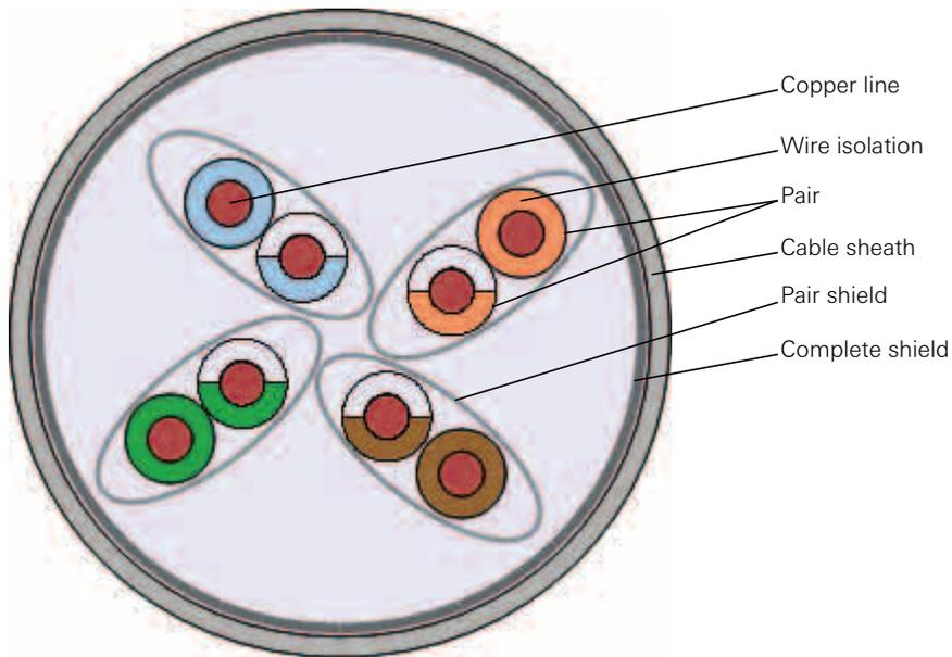
Figure 9.12: Structure of an S/FTP cable
