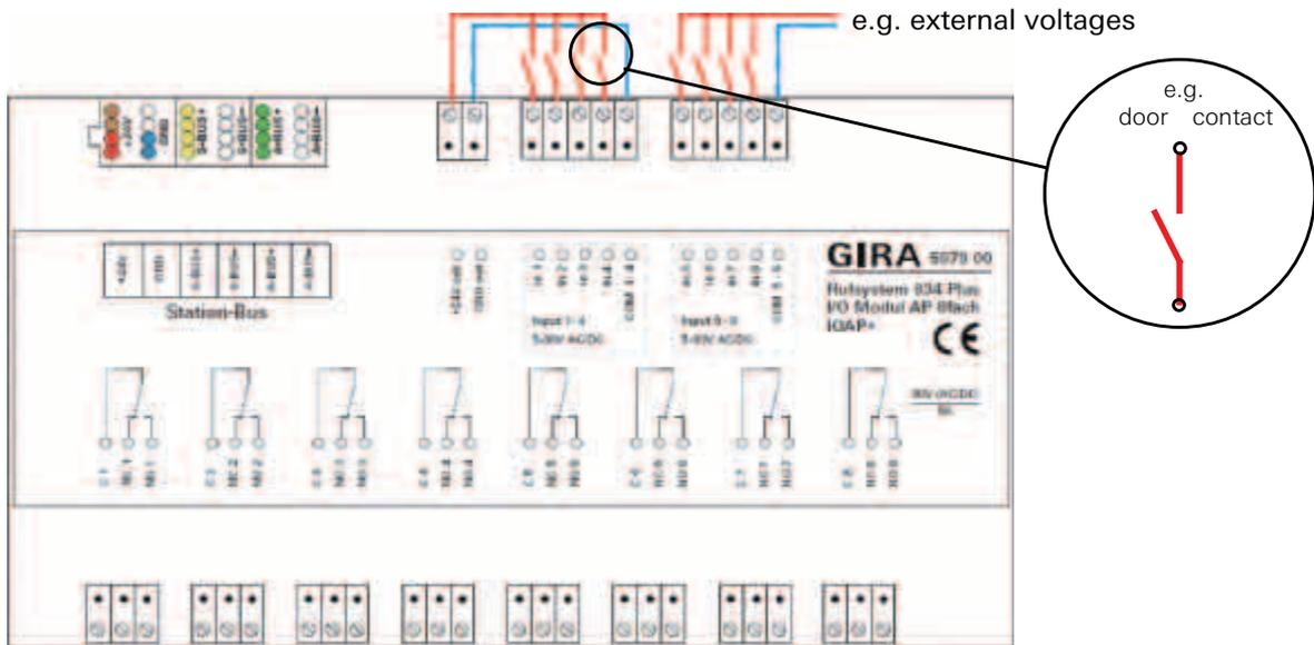
Figure 3.28: I/O module, 8-gang
