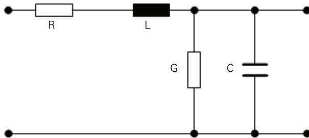
Figure 9.8: Equivalent circuit diagram for a short conductor length
