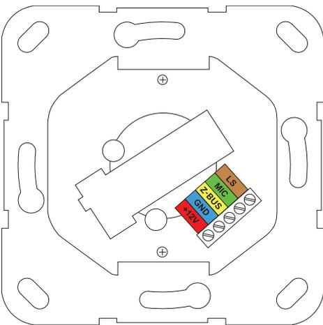
Figure 3.14: Connections of the pneumatic button
