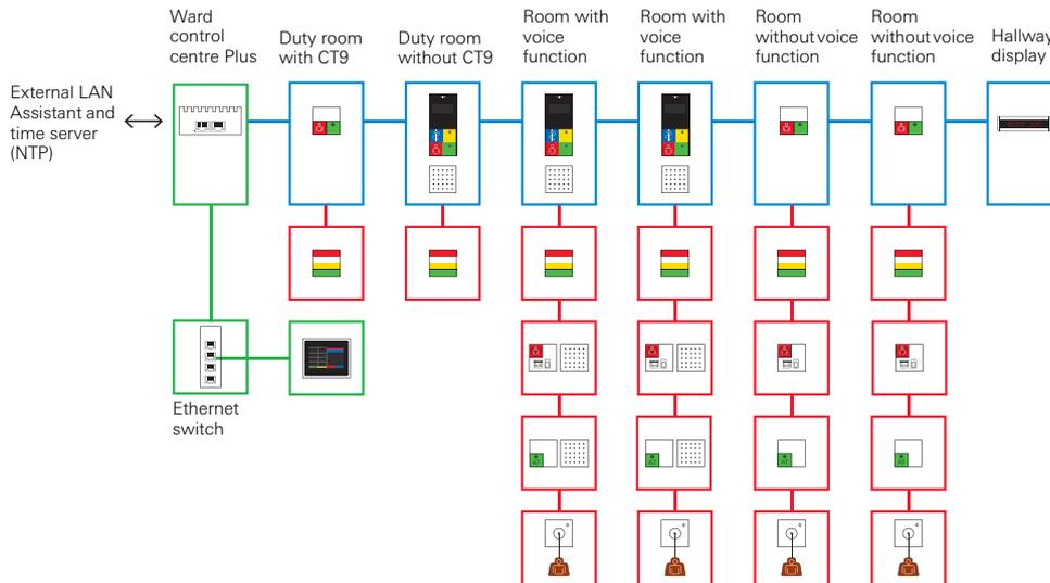
Figure 2.2: Small system with a ward control centre, switch and duty room terminal CT9
