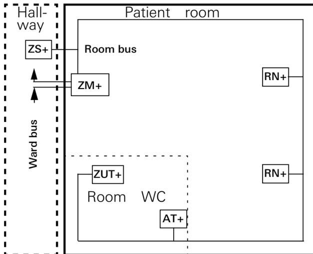
Figure 2.6: Block diagram for a twin bed room without voice function
