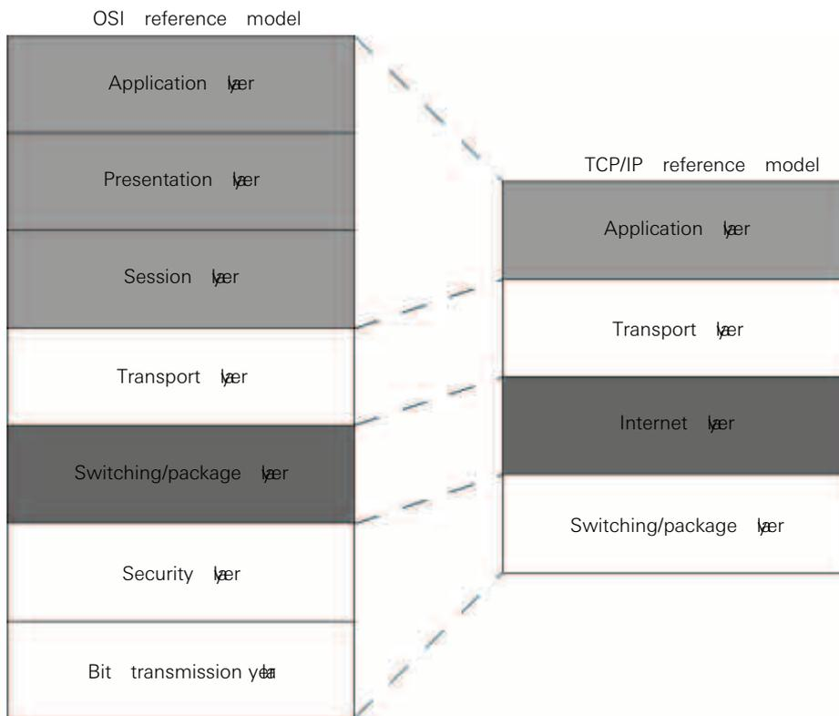
Figure 9.4: Block scheme of the TCP/IP reference model compared to the OSI model
