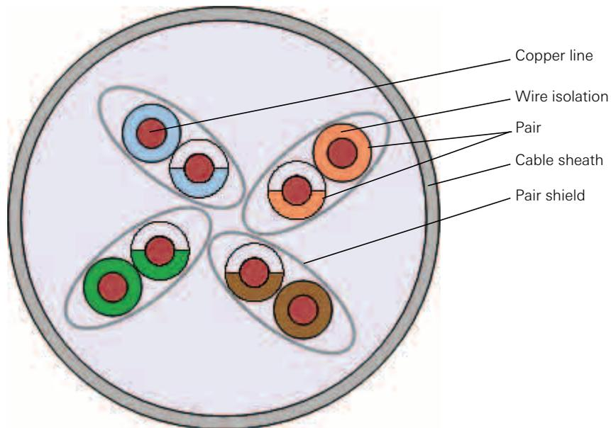
Figure 9.11: Structure of an FTP cable
