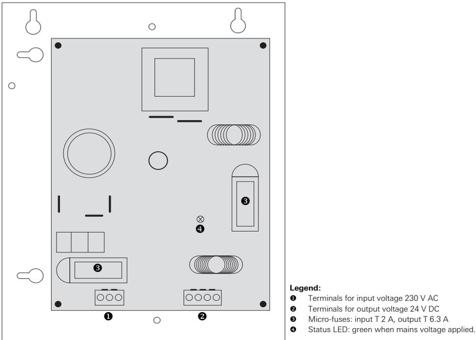
Figure 3.21: Device overview of power rectifier
