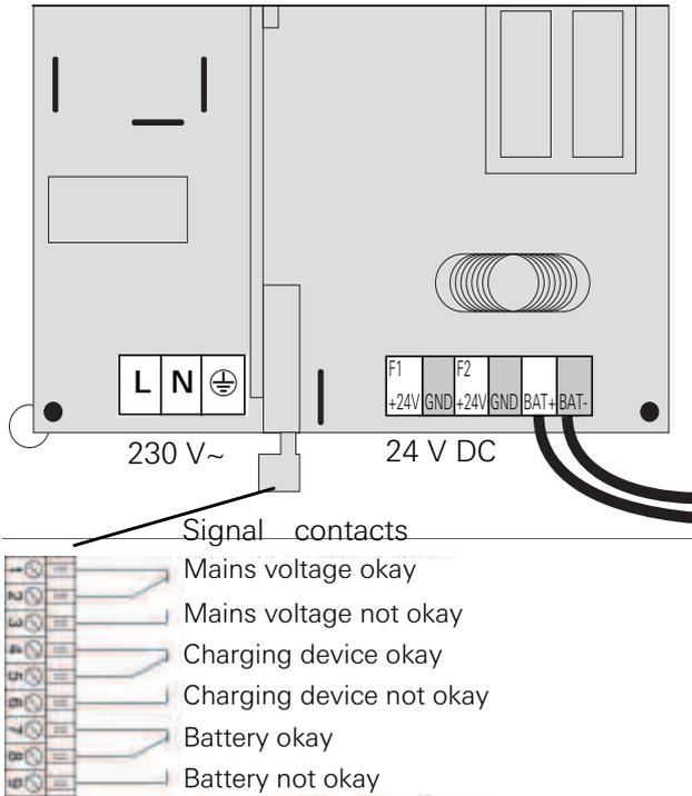
Figure 3.20: Connection of the power rectifier with UPS
