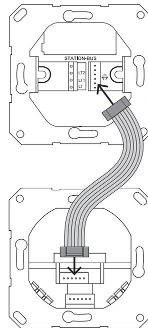
Figure 3.9: Connection of the voice module 5990 .. via flat ribbon cable to a voice-compatible room device.
