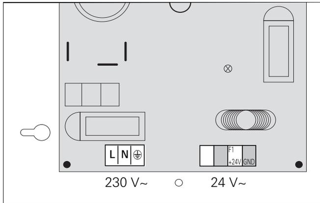
Figure 3.22: Connections of power rectifier without UPS
