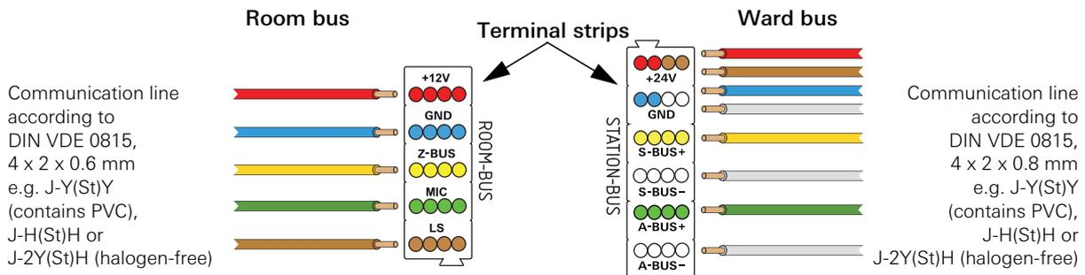
Figure 2.1: Colour coding of the connection terminals and recommended cable material
