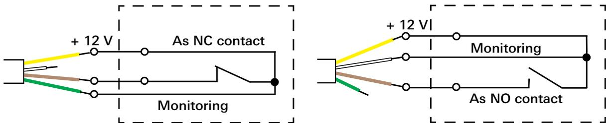
First connect the open end as shown, then insert the RJ11 plug of the connection cable into the diagnostic socket of the call button (5906.. or 5907..).
