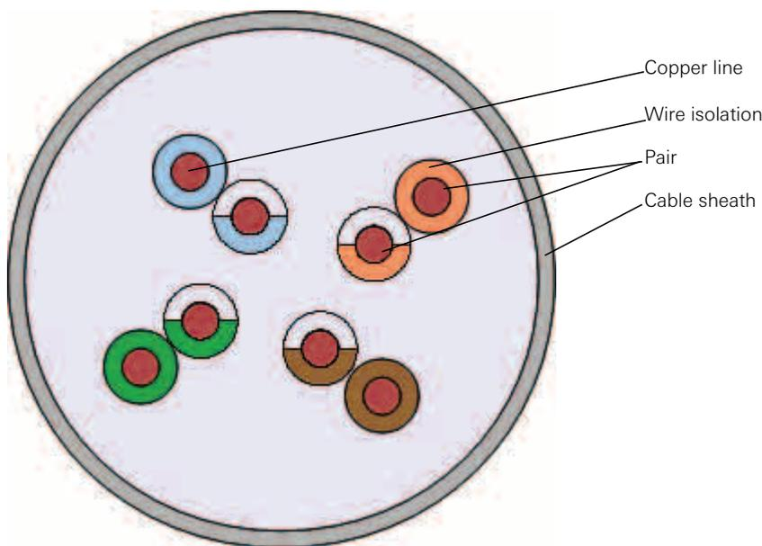
Figure 9.10: Structure of a UTP cable
