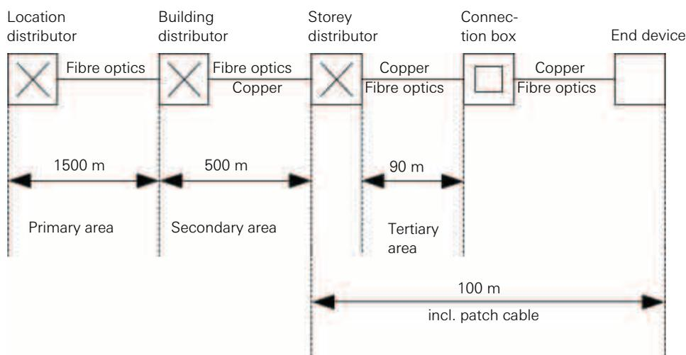
Figure 9.9: Structured cabling according to the ISO standard and European standard
