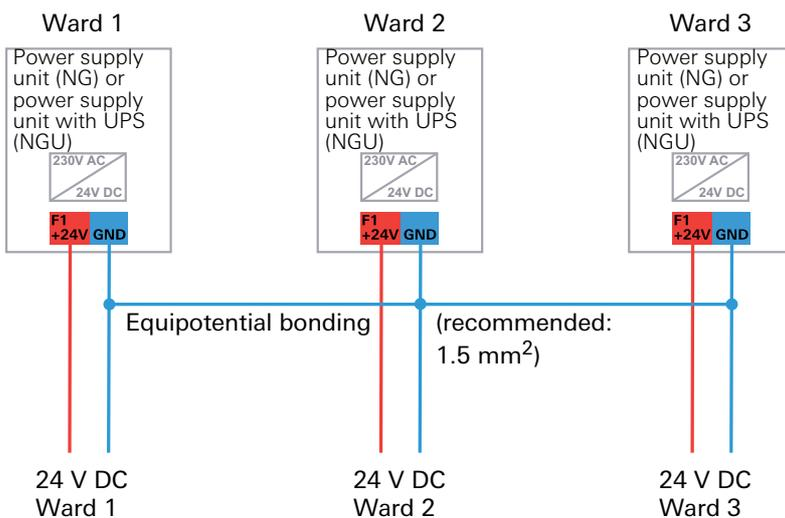
Figure 3.25: Equipotential bonding between the power supply units of a system
