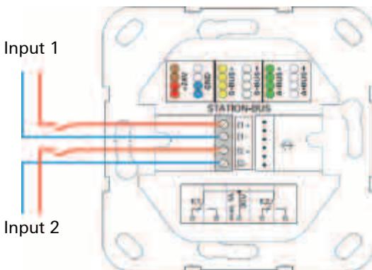
Figure 3.27: I/O module, 2-gang
