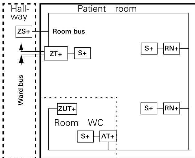
Figure 2.7: Block diagram for a twin bed room with voice function
