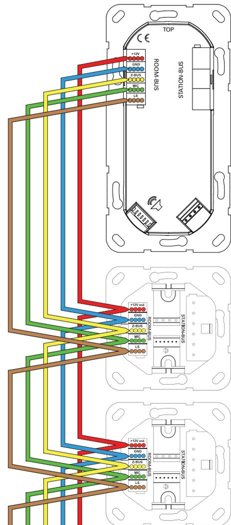
Figure 3.8: Colour coding of J-Y(St)-Y cable material on the room bus
