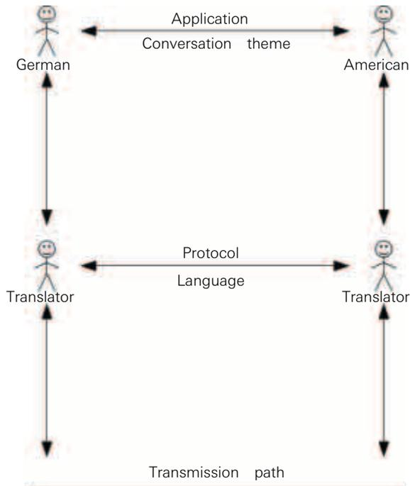
Figure 9.2: Example of a simple layer model
