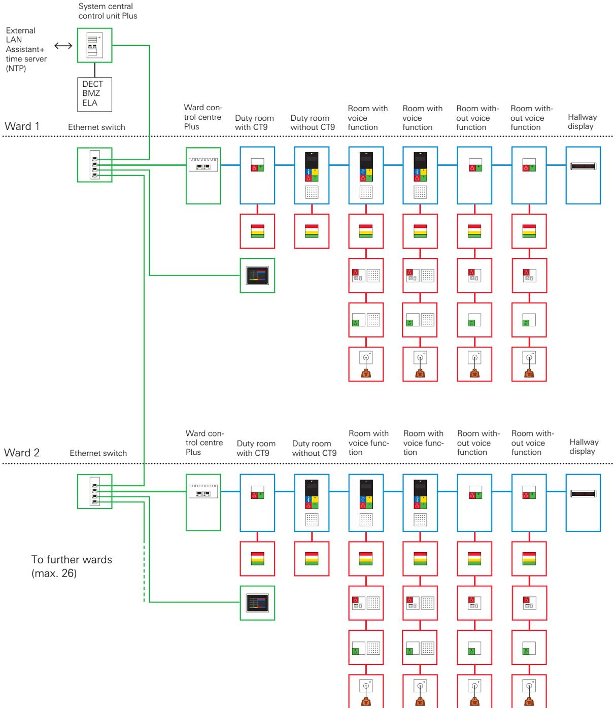
Figure 2.3: Example of system design for a large system
