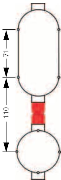
To ensure an optimal appearance, the distance between the terminal and the voice module should be implemented as shown. With the products ZT+ (Order No.: 5925 ..) and DZT+ (Order No. 5929: ..), flush-mounted boxes (1- and 2-gang) as well as a suitable spacer are included.
