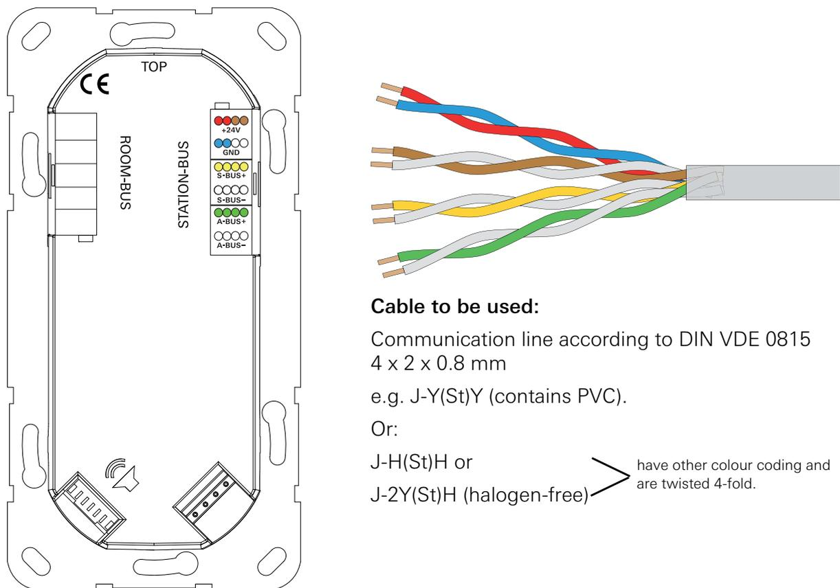
Figure 3.15: Colour coding of J-Y(St)-Y cable material on the ward bus
