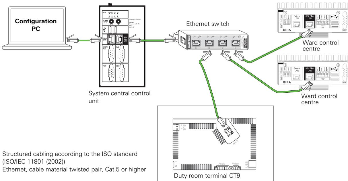
Figure 3.31: Connection of network components at system level (large system)
