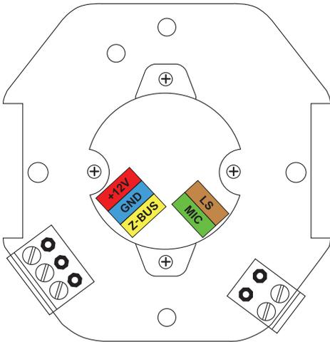
Figure 3.13: Connections of the pull-cord button
