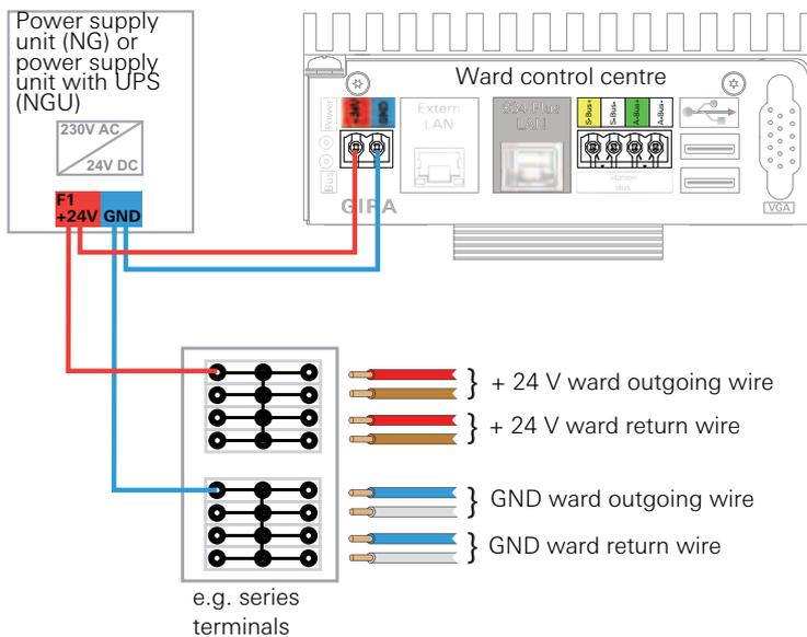
Figure 3.24: Outgoing and return wire of power supply to series terminal
