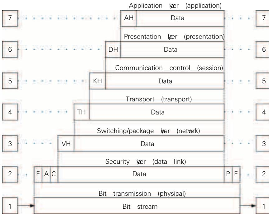
Figure 9.3: Graphic display of the OSI layer model
