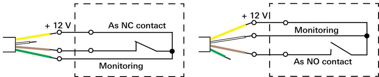
Figure 3.12: Diagnostic connection cable
