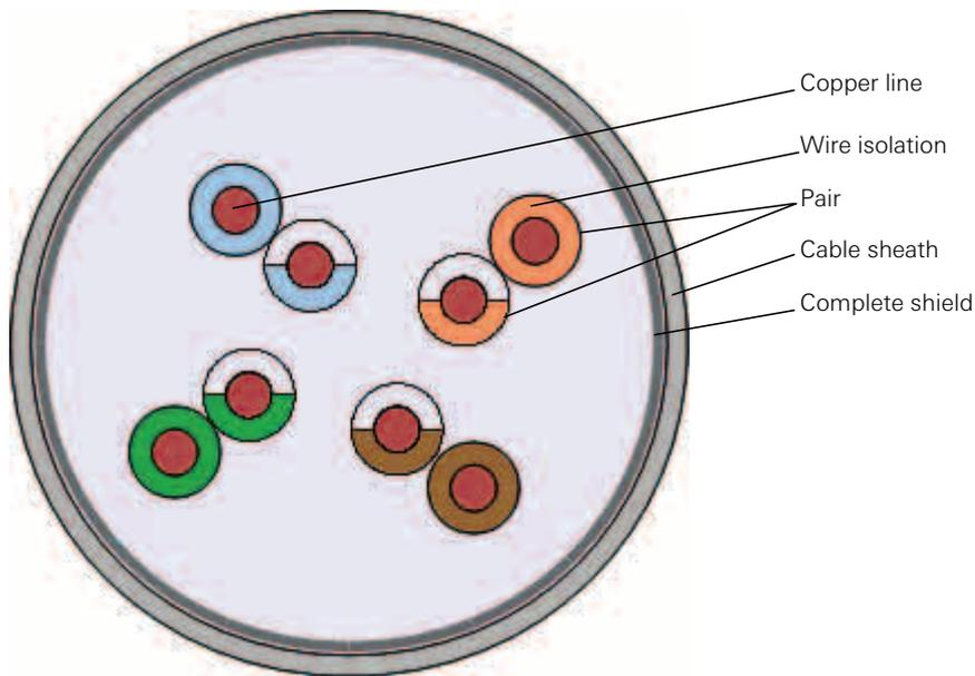
Figure 9.13: Structure of an S/UTP cable
