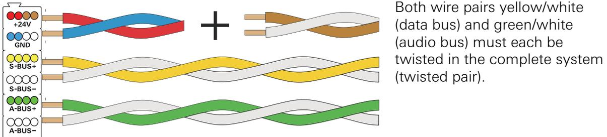
Figure 3.16: Use of 2 wire pairs for doubling of cross-section with power supply
