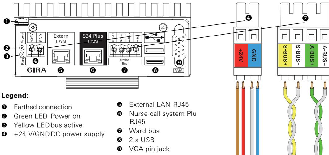
Figure 3.18: Ward control centre connections
